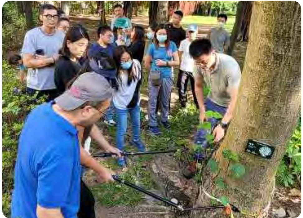
Trainees practising the use of a Sonic Tomograph to assess the internal condition of a tree trunk.
