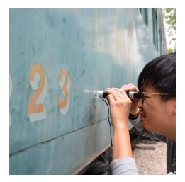
A conservator inspecting the paint coating on a train coach with a handheld microscope.
