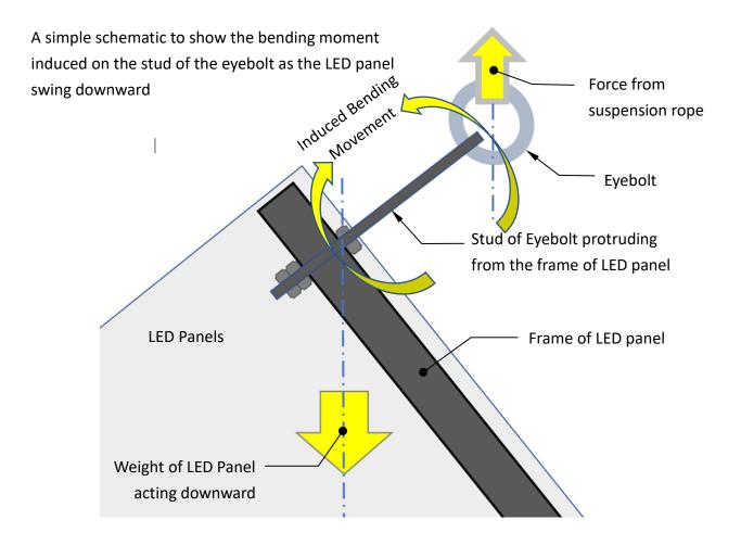
16.2 A total of 3 samples of the stud of the eyebolt, including the eyebolt from the broken suspension wire rope of the fallen LED panel were tested. The tensile strength of these studs were determined to be 840 MPa, 865 MPa, 846MPa which suggests that these studs were likely to be of Grade 8.8 (required minimum tensile strength of M12 Grade 8.8 bolt/stud is 830 MPa). No abnormality was observed in the breaking mode of these studs.
