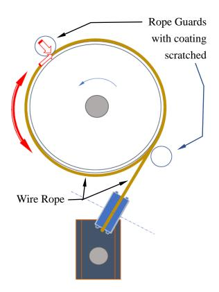
(f) Signs of scratching along the edges and walls of successive grooves on some of the winches were observed. Additional damage to the rope in the form of rope twist was induced by the slightly misaligned spooling guide rollers of the winch that further increased the stress imposed on the suspension wire ropes, and hence further reduced the fatigue resistance of the rope.
