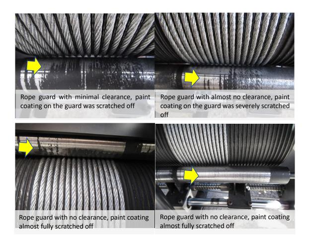
(e) The effects of rope guard(s) onto the rope are summarised in the following diagram.
