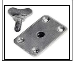
The boss plate is an M10 nut attached to a mild steel plate. Used in conjunction with an M10 thumbscrew it can be used (inverted) as an alternative to the stage screw. The boss plate fixes to the stage using four No. 8 wood screws.
