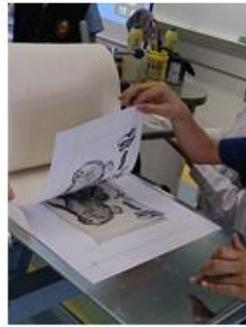
10. Making a print with a printmaking machine: Adjust the pressure of the printmaking machine. Place the polyester plate onto the machine and cover it with the moist printmaking paper. Then place a thick piece of cardboard and an etching blanket on top and make the print.
